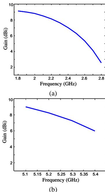
**Figure 8.** Simulated antenna gains against frequency for the proposed antenna in the
