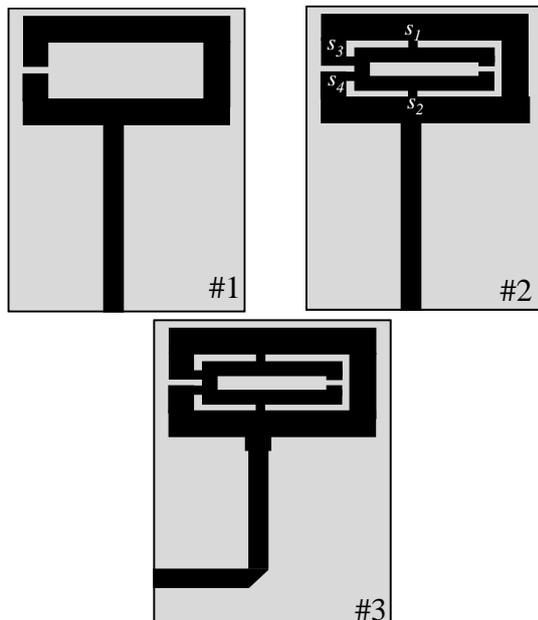
Figure 2. Design steps of the proposed antenna.
