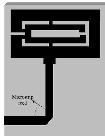
Figure 1. Proposed SRMA design (top view is shown).
