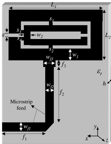
**Figure 4.** Proposed Multi-band SRMA design:  $s_1, s_2, s_3, s_4$  (metallic loadings:  $1 \times 1$ ),  $L_1=28, L_2=15, w_1=3.5, w_2=2, g=1, f_1=13, f_2=16.5, f_3=2, h=0.4$  (all in mm),  $\epsilon_r=4.4$ .
