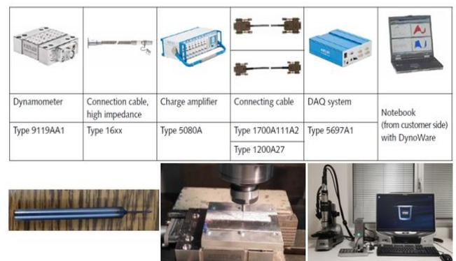
Figure 2 Test arrangement
