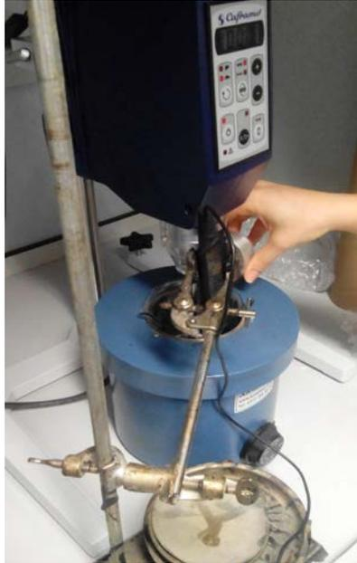
Fig. 2. Modification process by high shear mixer
