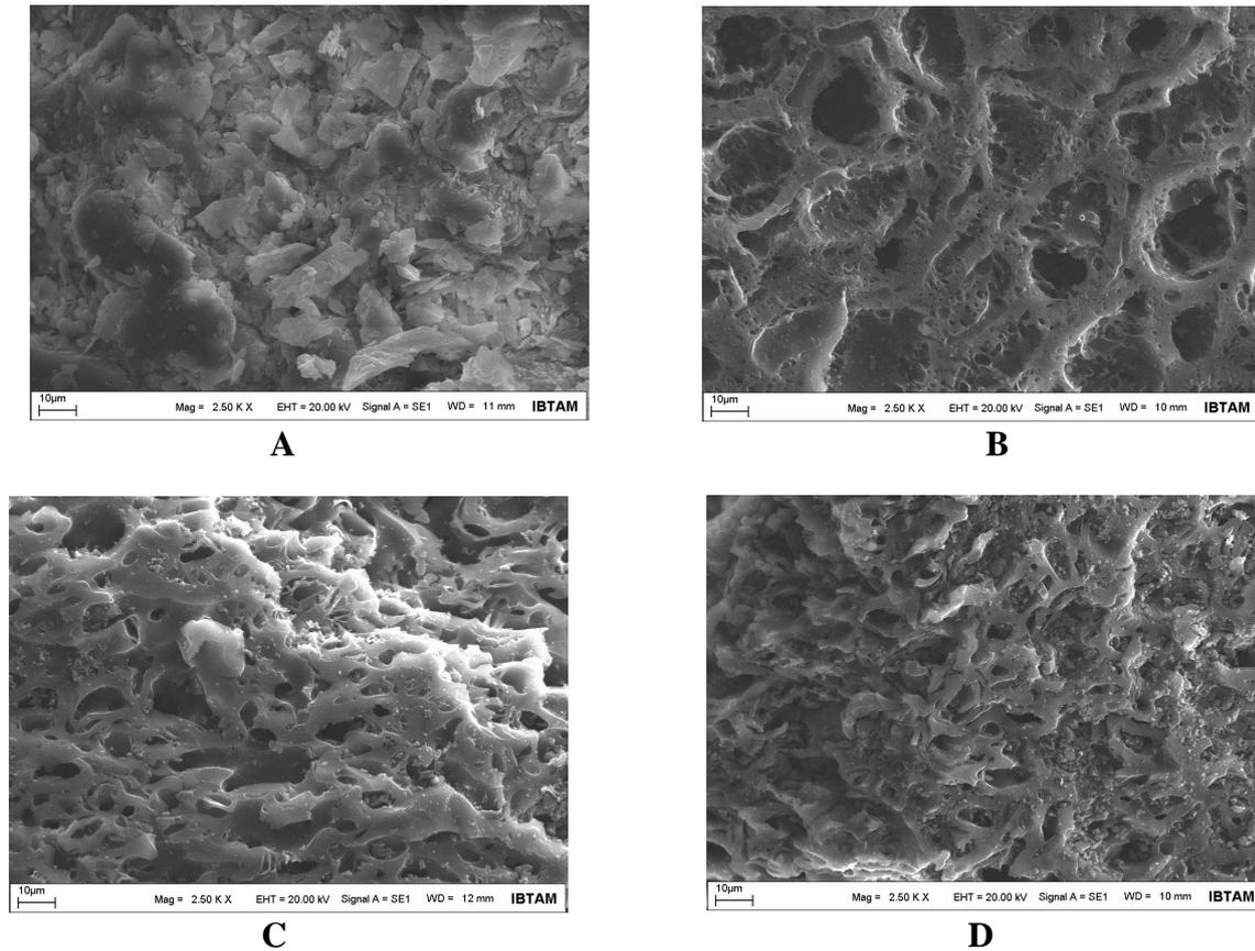
**Figure 4:** **A.** SEM image of raw pistachio shell **B.** Activated carbon sample at 600 °C 100 ml / min N<sub>2</sub> carbonization and at 800 °C with 100 mL / min CO<sub>2</sub> activation **C** Activated carbon sample at 500 °C 100 mL / min N<sub>2</sub> carbonization and at 800 °C with 100 mL / min CO<sub>2</sub> activation **D.** Activated carbon sample at 300 °C 100 mL / min N<sub>2</sub> carbonization and at 800 °C with 100 mL / min CO<sub>2</sub> activation.
