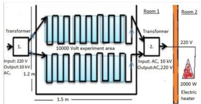
Figure 1a. The experiment setup.
