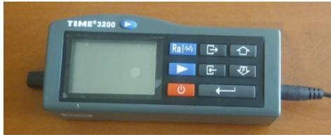
Figure 1. Surface Roughness Tester TIME 3200
