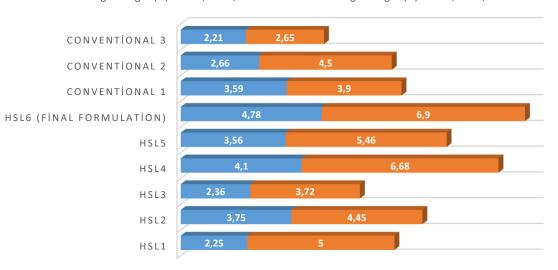
Figure 6: HS Strengths in Newton at sealing condition 1 and 2.
