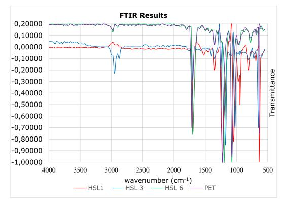
Figure 10: FTIR Result of HSL Formulations.
