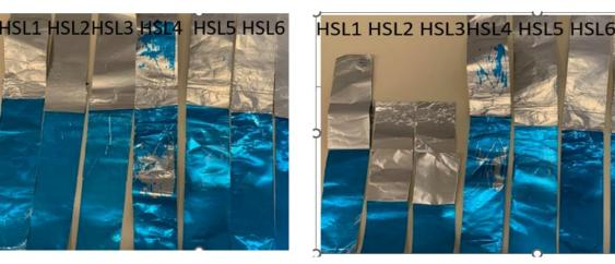
Figure 11: Block Test Result of Drawdowns at conditions 45 0C, 3 days, 45 kg & 20-25 °C, 1 week, 10 tons.
