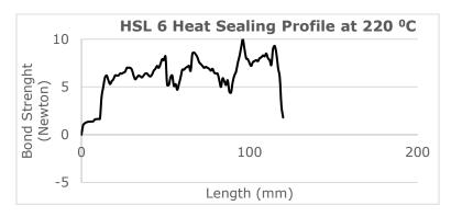
Figure 8: HSL 6 HS Profile at 220 °C.
