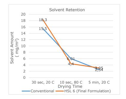
**Figure 12:** Residual solvent amounts [mg/m<sup>2</sup>].
