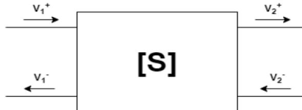
Figure 1. Illustration of a two-port circuit
