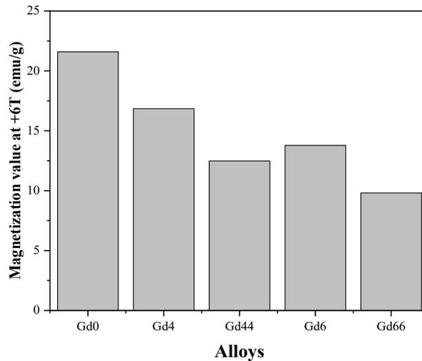
**Figure 6.** Comparison of saturation values of NiMnSGd alloys
