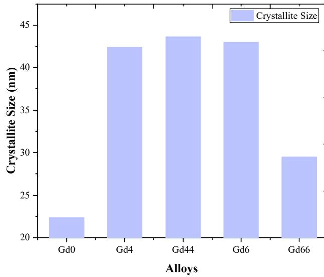
Figure 2. Comparison of crystal size of NiMnSn-Gd alloy
