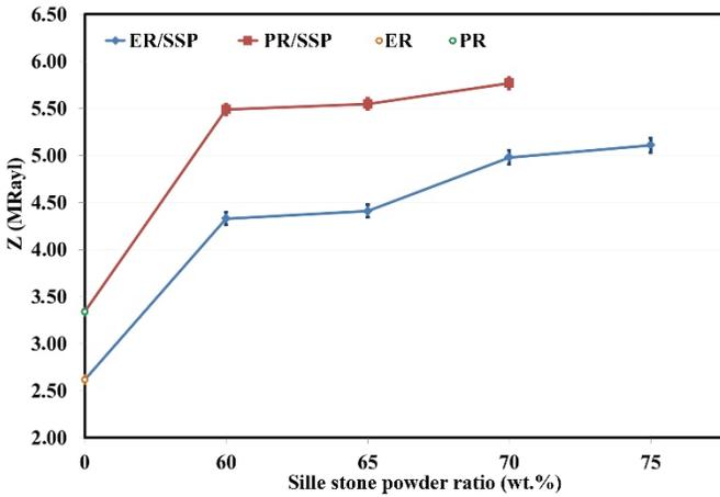
Figure 10 - Change in ER and PR different amounts of SSP acoustic impedance ( $Z$ ) values.
