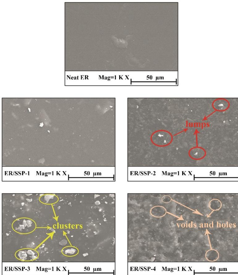
Figure 3 - SEM images of the ER/SSP composites (Magnification of 1.00 K X, 50 µm).
