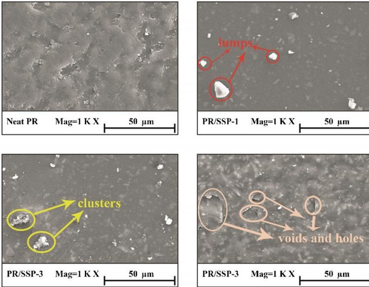
*Figure 4 - SEM images of the PR/SSP composites (Magnification of 1.00 K X, 50 μm).*
