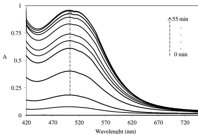
**Fig. 5.** The change in the absorbance of Epinephrine (EP) with time catalyzed by PEI-Co(II). [PEI-Co(II) = 60 mg, and EP = 2 mM, and  $H_2O_2$  = 46 mM at 30 °C].
