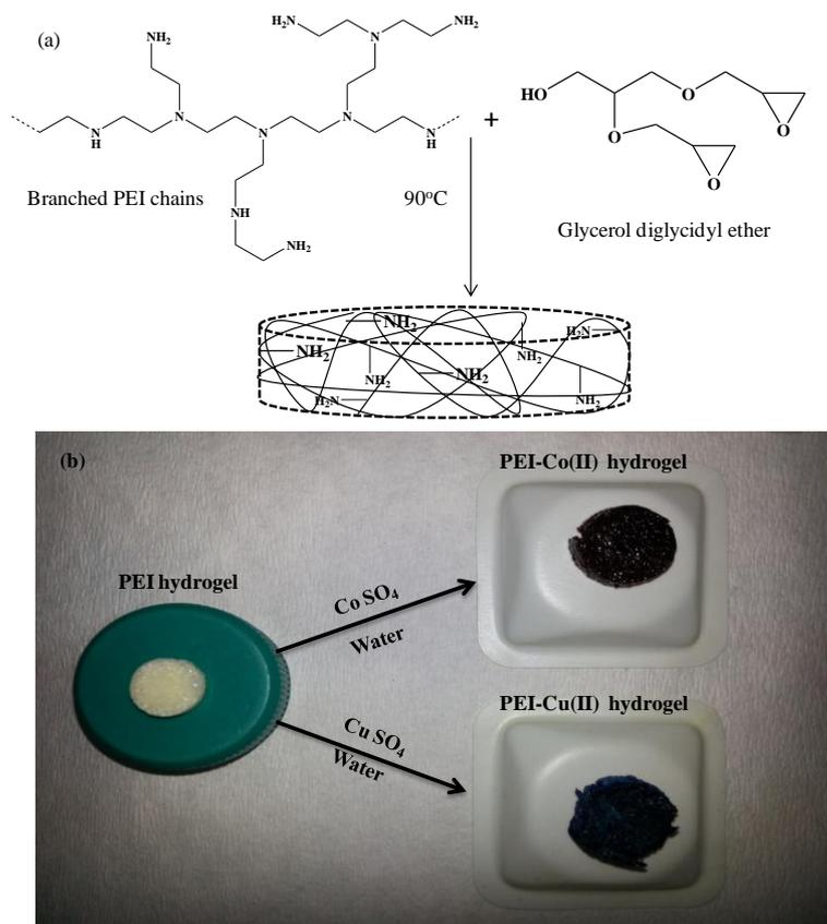
**Fig. 1.** (a) PEI hydrogel preparation, and (b) PEI hydrogels's complex formation with Co(II) and Cu(II) ions.
