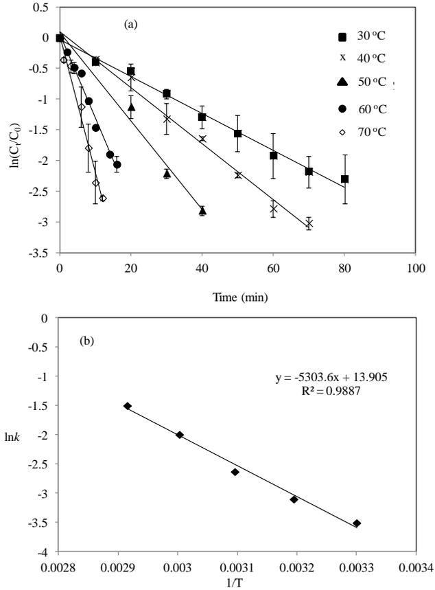
**Fig. 4.** a) The relationship between  $\ln(C_t/C_0)$  with time at different temperature, b) Arrhenius plot of  $\ln k$  versus  $1/T$  for the degradation of MO catalyzed by PEI-Cu(II).
