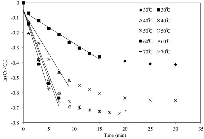
**Fig. 7.** The effect of temperature on  $\ln(C_t/C_0)$  with time.
