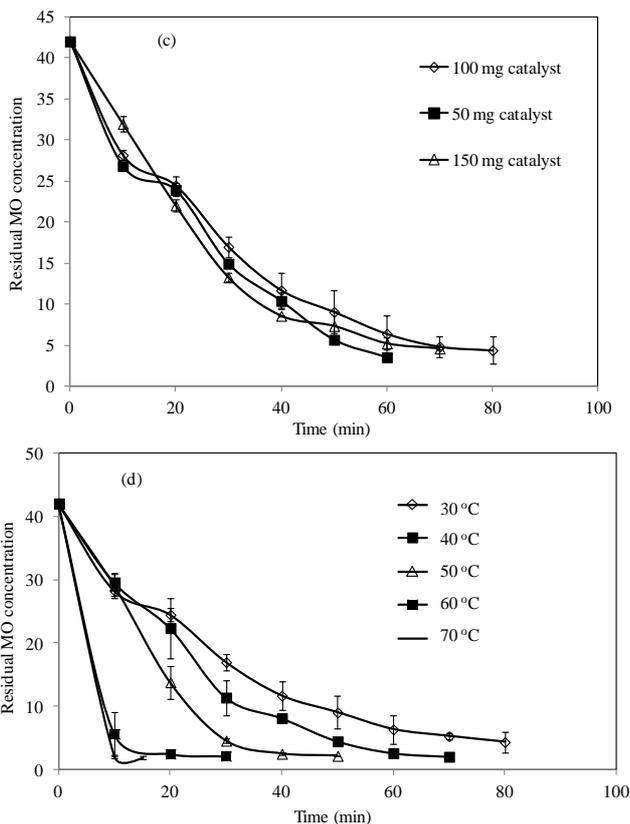
**Fig. 3.** Residual MO concentration versus time for the degradation of MO catalyzed by PEI-Cu(II) hydrogel composite with a) various  $H_2O_2$  concentration, b) various concentration of MO, c) various amount of catalyst, d) at different temperatures.
