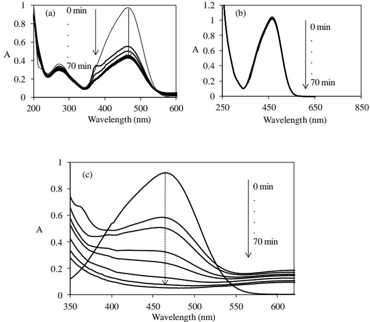
**Fig. 2.** UV-Vis spectra of degradation of methyl orange with a) PEI-Cu(II) hydrogel composite as a catalyst without  $H_2O_2$ , b)  $H_2O_2$  without catalyst, c) PEI-Cu(II) hydrogel composite as catalyst and  $H_2O_2$  as an oxidant.
