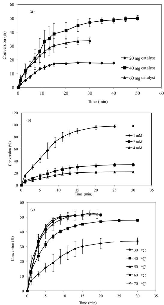
**Fig. 6.** Epinephrine conversion in the presence a) different amount of PEI-Co(II) catalyst, b) different concentration of epinephrine (EP), c) at different temperatures.
