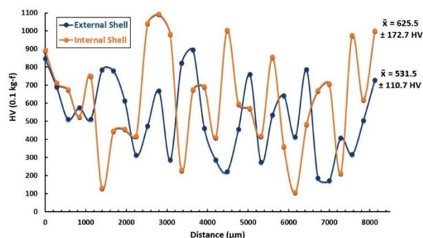
**Figure 8.** The Vickers microhardness results of the *A. anatina* shell samples
