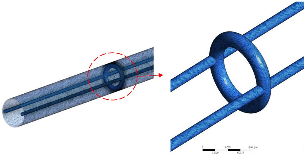
**Figure 6.** Mesh quality of pipe and circular turbulator.
