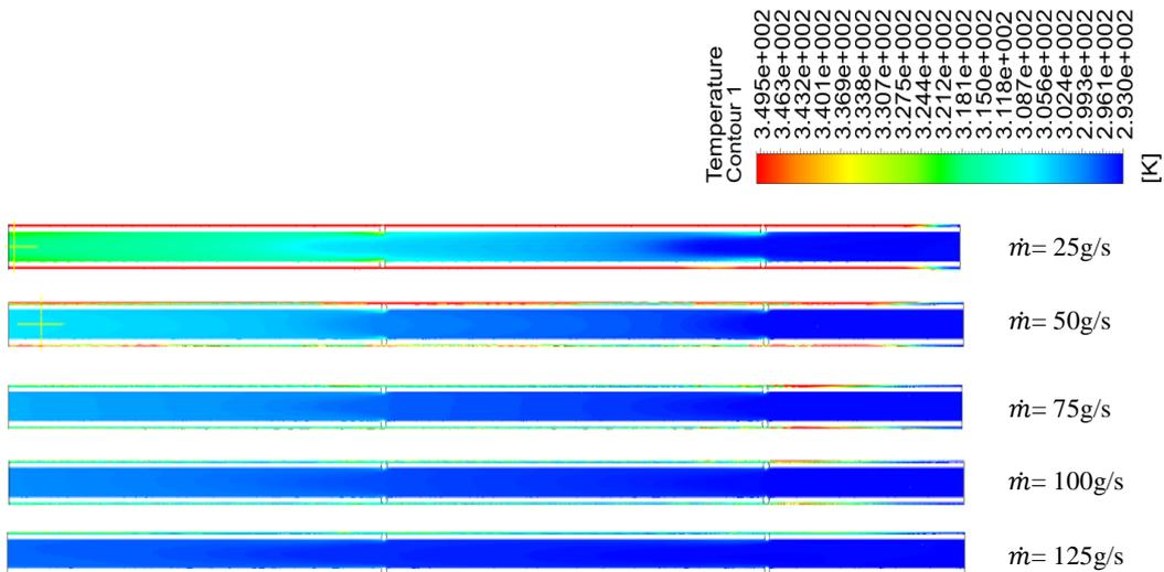
**Figure 11.** Temperature contours for pipe inserts at different mass flow rates.
