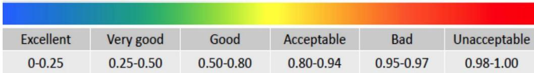
**Figure 4.** Mesh skewness spectrum and the scales for the Skewness criterion.
