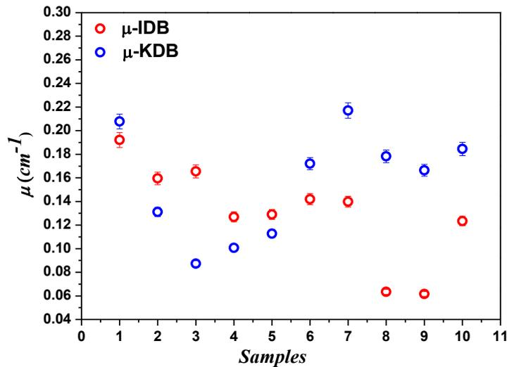
**Figure 4.** Gamma-rays Linear attenuation coefficients versus samples
