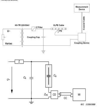
Figure 2. Circuit diagrams of the PD test system
