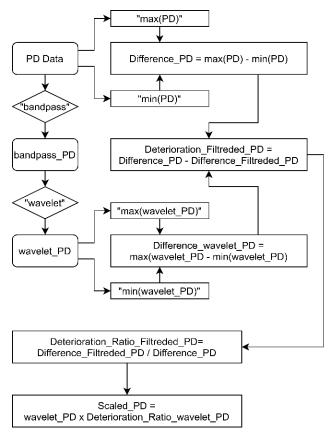
Figure 4. Flowchart of the proposed algorithm
