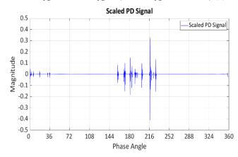
Figure 6. Scaled partial discharge signal.
