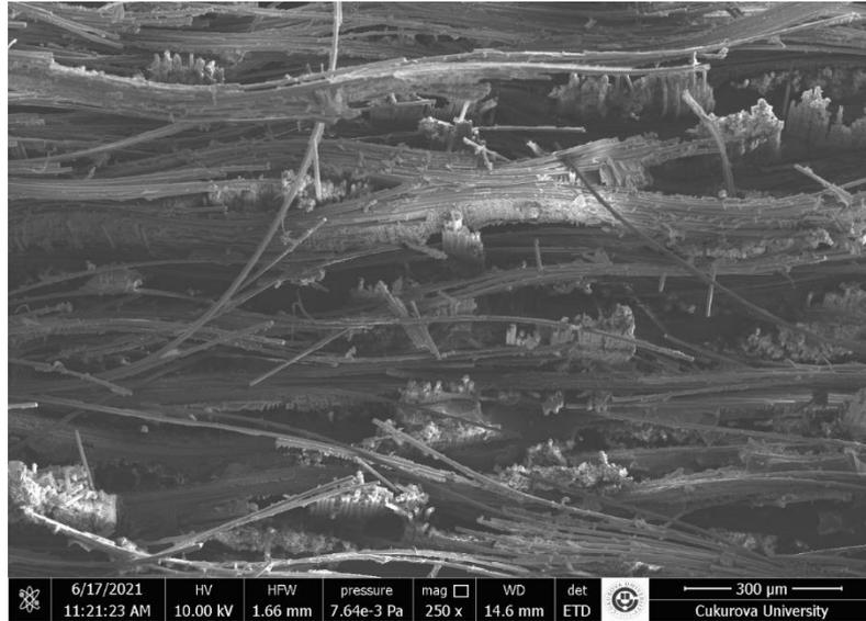
**Figure 19.** After Flexural Test SEM images G10
