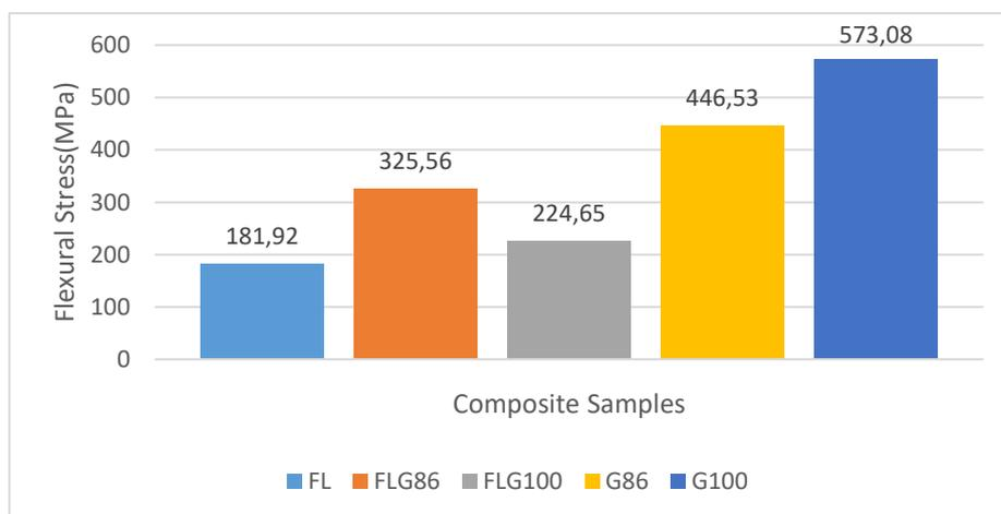
**Figure 9.** Three-point bending test results
