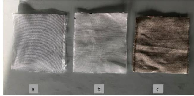
**Figure 1.** Fabric samples: a) Glass fiber (86 gr/m<sup>2</sup>) b) Glass fiber (100 gr/m<sup>2</sup>) c) Flax
