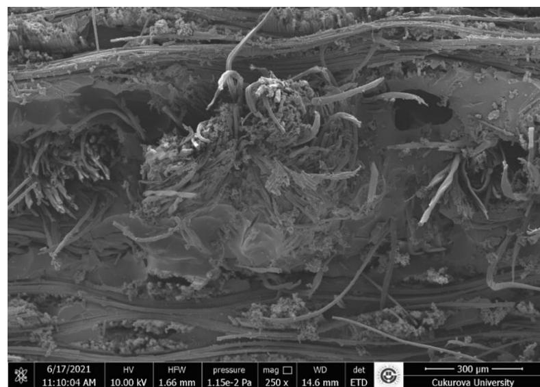
**Figure 21.** After Flexural Test SEM images of FLG100
