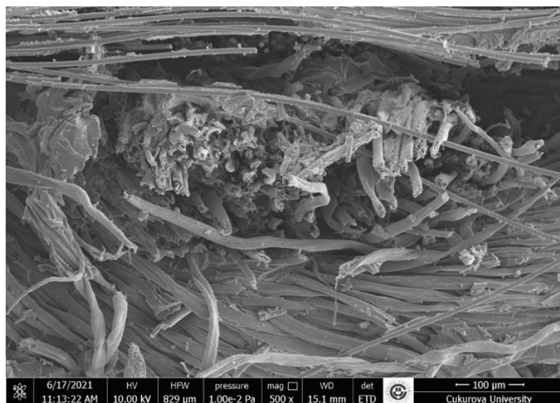
*Figure 16. After Tensile Test SEM images of FLG100*
