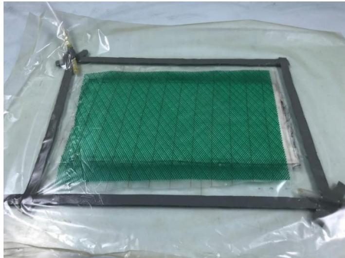
*Figure 2. Vacuum assisted resin transfer molding process*
