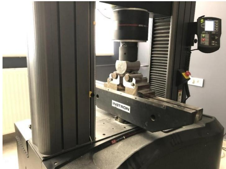
**Figure 5.** Three-point bending testing machine
