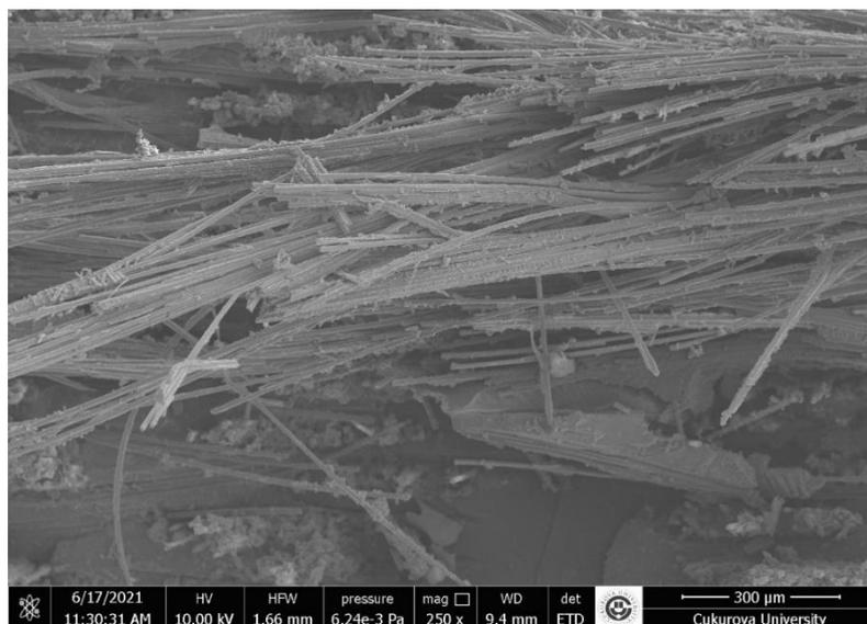
*Figure 13. After Tensile Test SEM images of G86*
