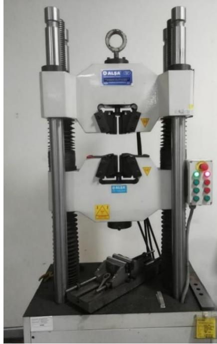
**Figure 4.** Tensile testing machine
