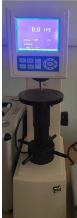
**Figure 6.** Rockwell hardness test machine
