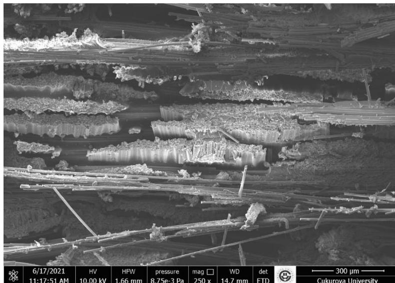
*Figure 18. After Flexural Test SEM images of G86*
