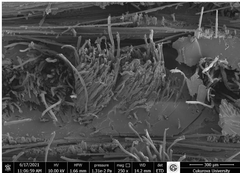
**Figure 20.** After Flexural Test SEM images of FLG86
