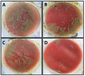
3. Cu<sub>2</sub>O gels in order of increasing Figure concentrations. (A) 0.1 g Cu<sub>2</sub>O, (B) 0.2 g Cu<sub>2</sub>O, (C) 0.3 g Cu<sub>2</sub>O, (D) 0.4 g Cu<sub>2</sub>O.
