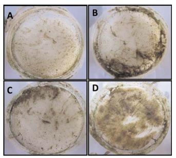
Figure 2. ZnO gels in order of increasing concentrations. (A) 0.1 g ZnO, (B) 0.2 g ZnO, (C) 0.3 g ZnO, (D) 0.4 g ZnO.
