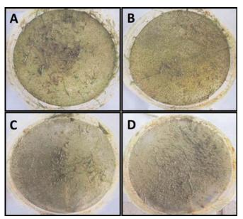
Figure 6. KS gels in order of increasing concentrations. (A) 0.5 M KS , (B) 1 M KS, (C) 2 M KS, (D) 4 M KS.
