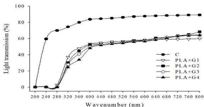
**Figure 1.** Effect of bovine gelatin thickness on light transmission values of bi-layer films
