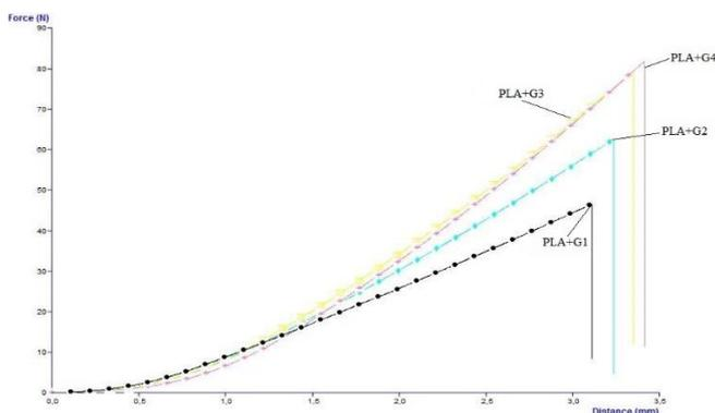
**Figure 3.** Puncture force and distance curves of bi-layer films.
