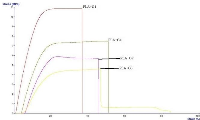
**Figure 2.** Stress vs strain curves of bi-layer films
