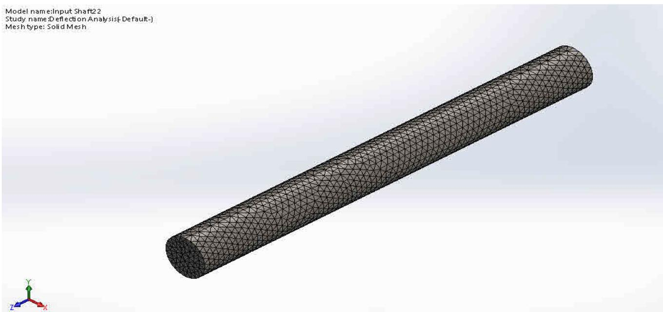
**Fig 2.** Mesh visualization of the sun gear shaft model
