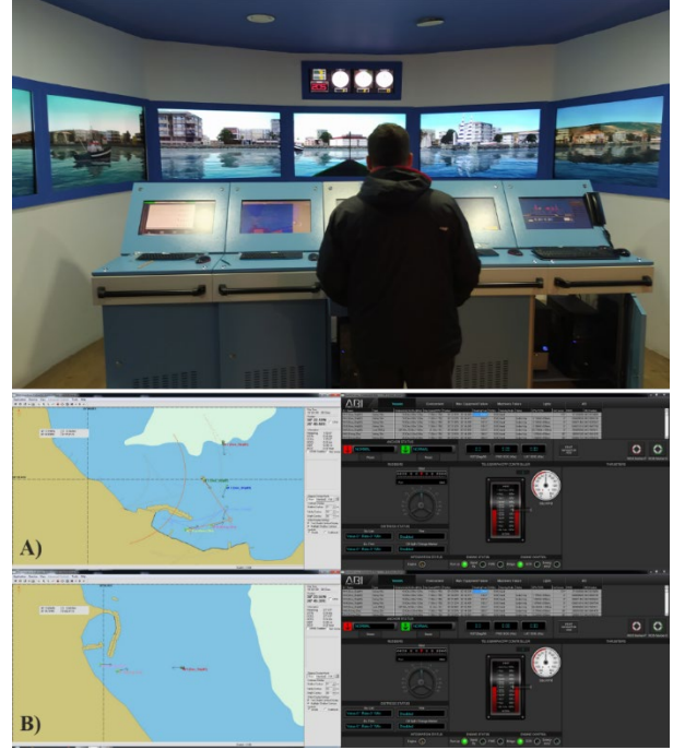
Figure 1. ARI (Applied Research International, Version 1.0) bridge operation simulator and port navigation for İskele and Çeşmealtı fishing ports in the simulator
