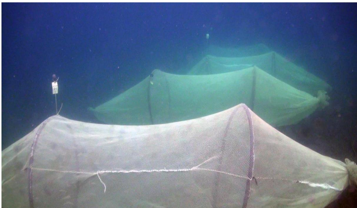
**Figure 2:** The settlement of codend covers were used as an observation cage during the experiments (Underwater video recordings were performed by F. Ozan Düzbastilar)
