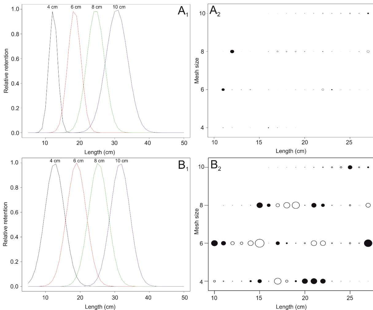
**Figure 3.** Selectivity curves and deviance residual plot of gillnets and trammel nets. (A: Gillnet; B: Trammel Net; 1: Selectivity curve ; 2: Deviance residual plot)
