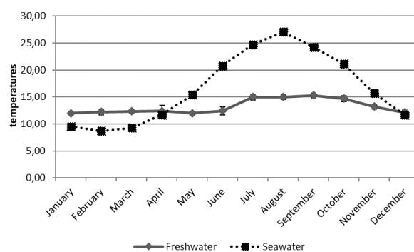
**Figure 1.** Yearly temperature records of freshwater re-circulating aquaculture system and marine cages. The lowest sea temperatures were recorded as 6.5°C in marine cages and 11.97°C in RAS unit. The highest temperatures were recorded as 29°C in marine cages and 15.28°C in RAS unit.
