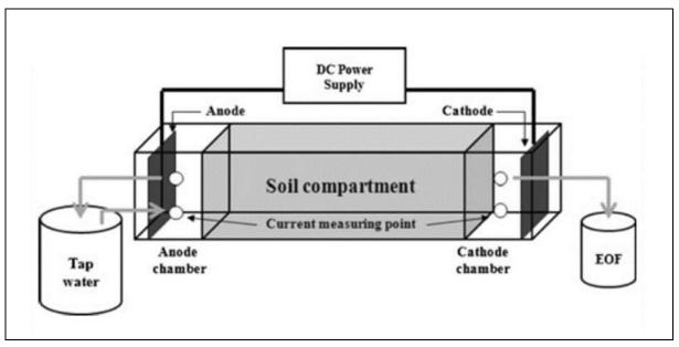
Figure 5. Schematic of an EK remediation system [7].
