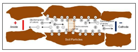
Figure 4. Transport mechanism of electrokinetic restoration [29].
