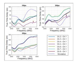
Figure 5. First block TTD test results.
