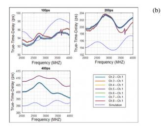
Figure 6. (a) First level of second block TTD test results. (b) Second level of second block TTD test results.
