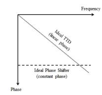
Figure 2. Comparison between TTD and phase shifter.
