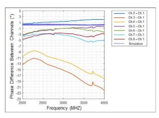
Figure 7. Phase difference test results between channels.
