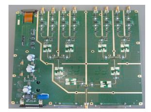
Figure 4. Manufactured beamforming PCB.
