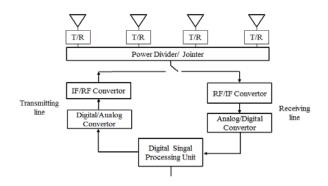
Figure 1. Block diagram of analog beamforming structure.
