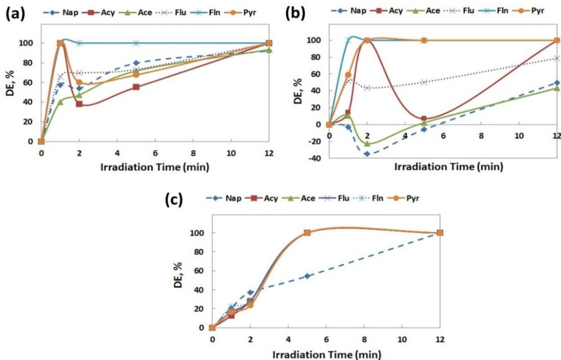
Figure 4. Degradation diagrams associated with the simulated solar irradiated treatments; Xe treatment (a), Xe/TiO<sub>2</sub> treatment (b), Xe/H<sub>2</sub>O<sub>2</sub> treatment (c)
