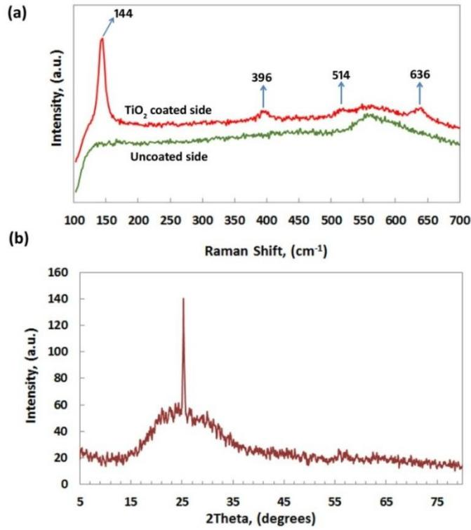
Figure 1. Raman spectra of glass surfaces (a) and XRD pattern of TiO<sub>2</sub> coated surface (b)
