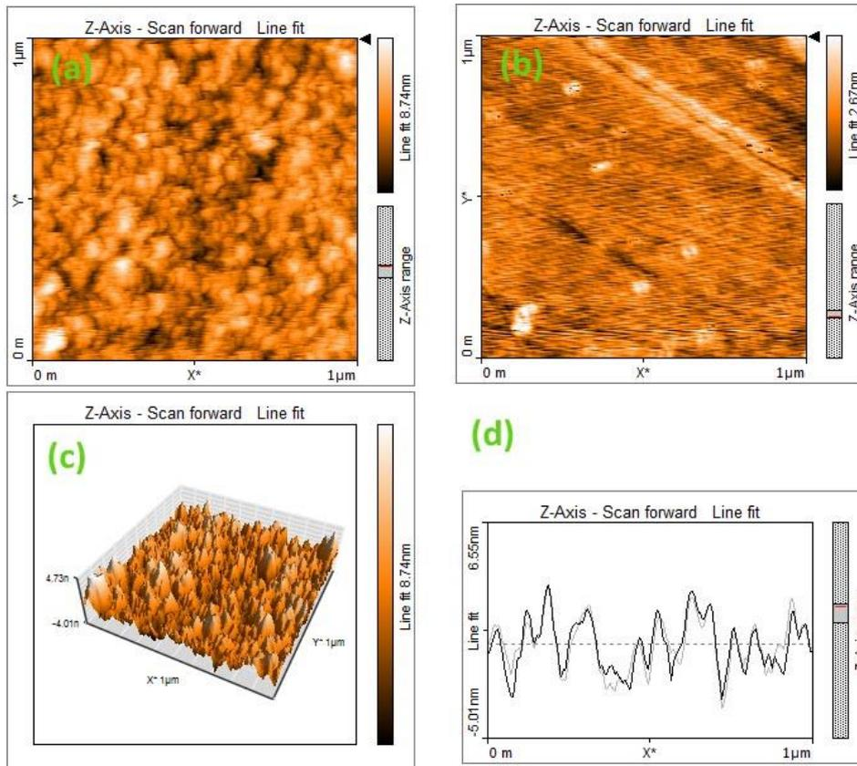
Figure 2. AFM images of Pilkington Activ™ glass in (a, b) a top-down view, (c) a topographical view, (d) sectional view for active and bar surfaces, respectively
