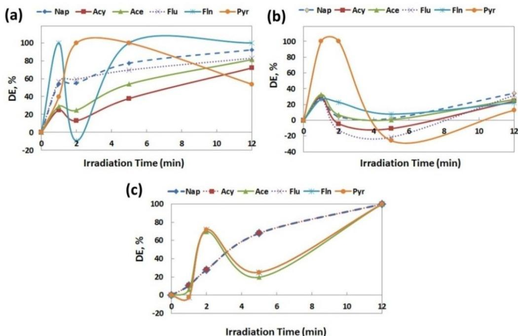
Figure 3. Degradation diagrams associated with UV-C irradiated treatments; UV-C treatment (a), UV-C/TiO<sub>2</sub> treatment (b), UV-C/H<sub>2</sub>O<sub>2</sub> treatment (c)
