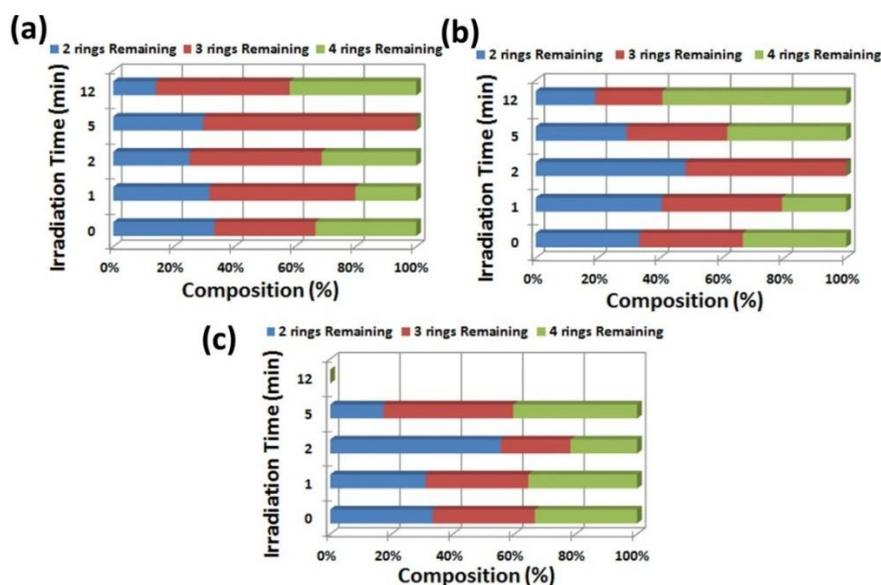
Figure 6. Remaining concentration composition of PAHs categorized according to their ring sequences for UV-C treatment (a), UV-C/TiO<sub>2</sub> treatment (b), and UV-C/H<sub>2</sub>O<sub>2</sub> treatment (c)
