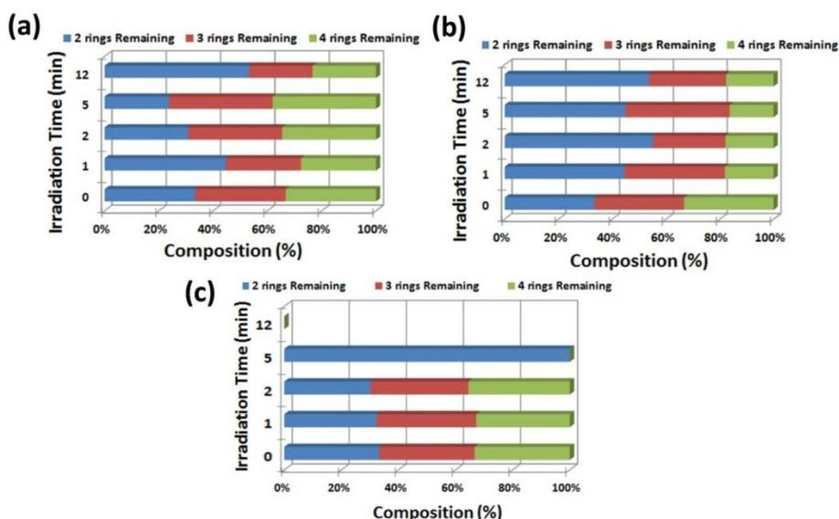
Figure 7. Remaining concentration composition of the PAHs categorized according to their ring sequences for Xe treatment (a), Xe/TiO<sub>2</sub> treatment (b), and Xe/H<sub>2</sub>O<sub>2</sub> treatment (c)
