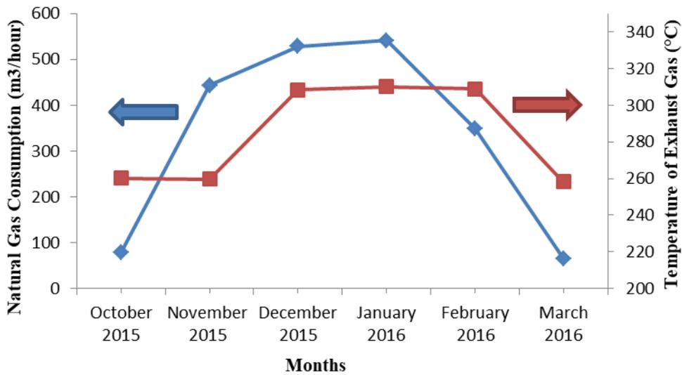
**Figure 2.** Natural gas consumptions and temperatures of exhaust gas of the boiler
