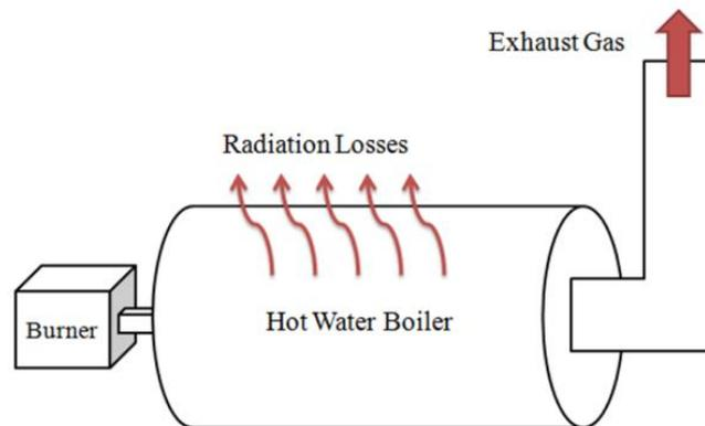
**Figure 1.** Schematic diagram and energy losses of the hot water boiler
