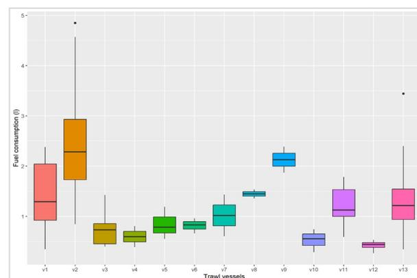
**Figure 2.** Box plot showing the fuel use intensity of each trawl vessel investigated
