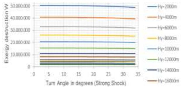
**Figure 8.** Variation of the exergy destruction with turn angles in degrees (strong shock) for  $Ma=5$  and different altitudes.
