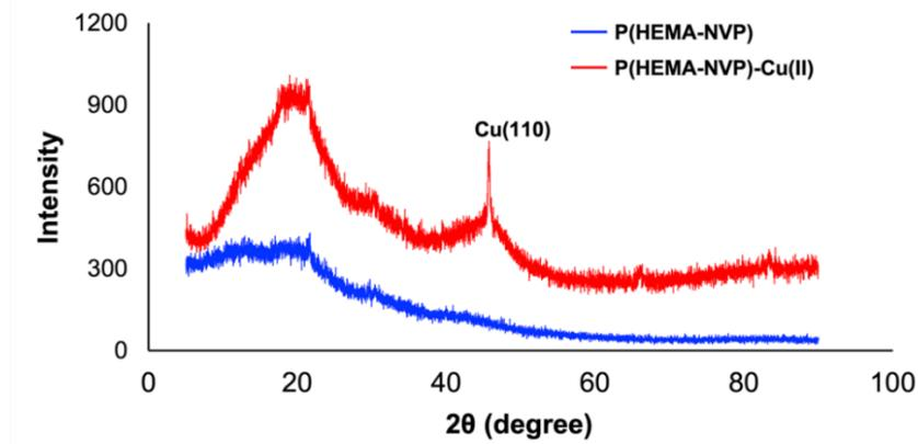
**Figure 4.** XRD images of the *P(HEMA-NVP)* and *P(HEMA-NVP)-Cu(II)* cryogels.
