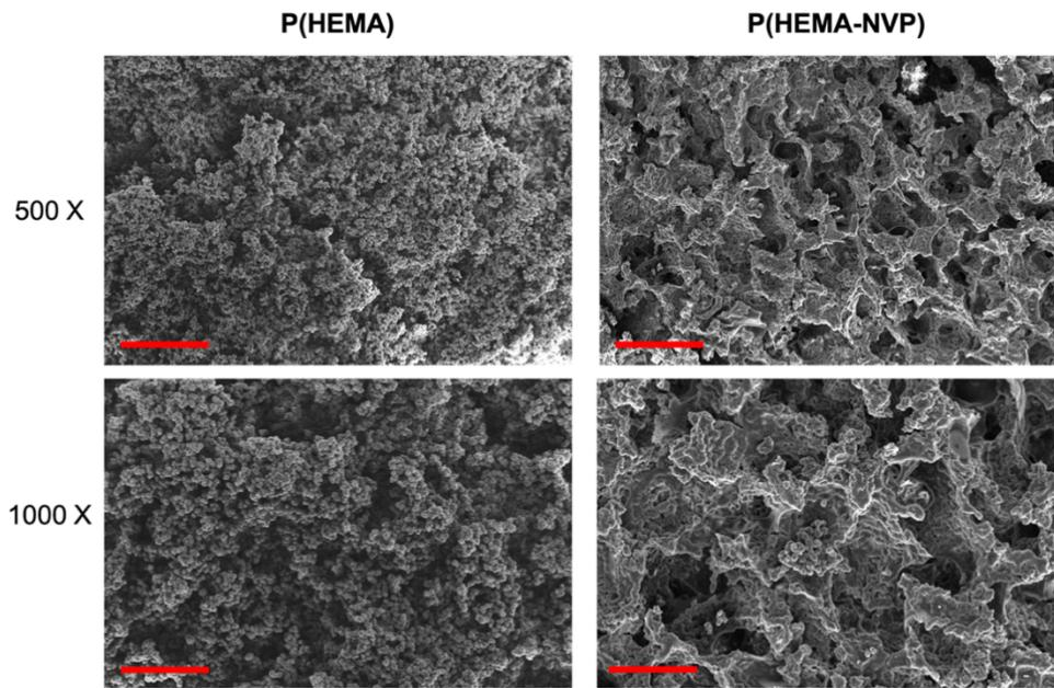
**Figure 3.** SEM images of P(HEMA) and P(HEMA-NVP) cryogels. Scale bar: 100  $\mu\text{m}$  for  $\times 500$ ; and 50  $\mu\text{m}$  for  $\times 1000$ .
