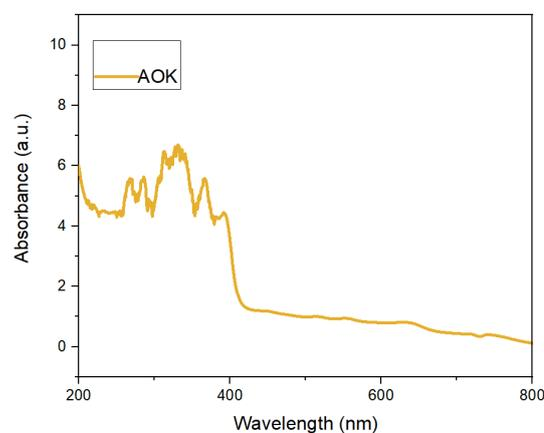
**Figure 11** Absorption versus wavelength of organic brown lens
