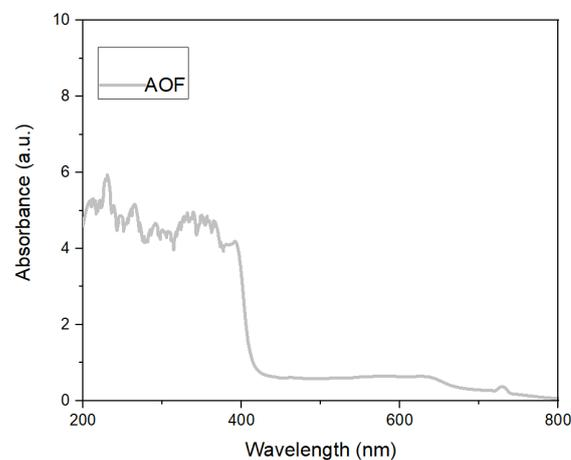
**Figure 12** Absorption versus wavelength of organic smoked lens
