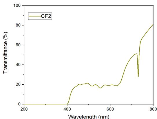
**Figure 3** Wavelength versus light transmittance plot of smoked mineral lens
