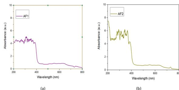
**Figure 2** (a) Absorbance plot of Mineral Smoked lens versus wavelength on the horizontal axis, (b) absorbance plot on the vertical axis
