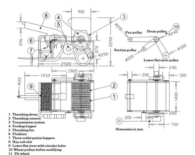
Figure 1. Threshing machine before modification.
