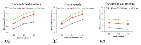
Figure 4. (A). Effect of drum speeds on threshing efficiency at concave hole diameters; (B). Effect of concave hole diameters on threshing efficiency at drum speeds; (C). Effect of feed rates on threshing efficiency at concave hole diameters.
