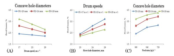
Figure 5. (A) Effect of drum speeds on seed losses at concave hole diameters; (B). Effect of concave hole diameters on seed losses at drum speeds; (C) Effect of feed rates on seed losses at concave hole diameters.
