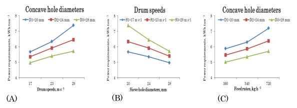
Figure 7. (A). Effect of drum speeds on the power requirements at concave hole diameters; (B)Effect of concave hole diameters on the power requirements at drum speeds; (C) Effect of feed rates on the power requirements at concave hole diameters.
