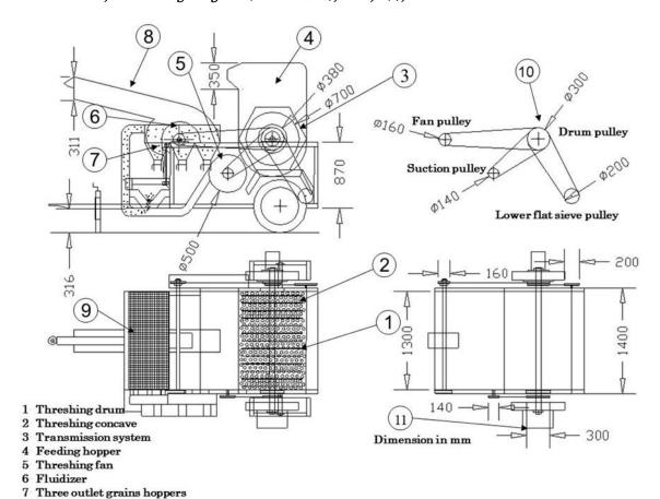
Figure 2. Threshing machine after development.
