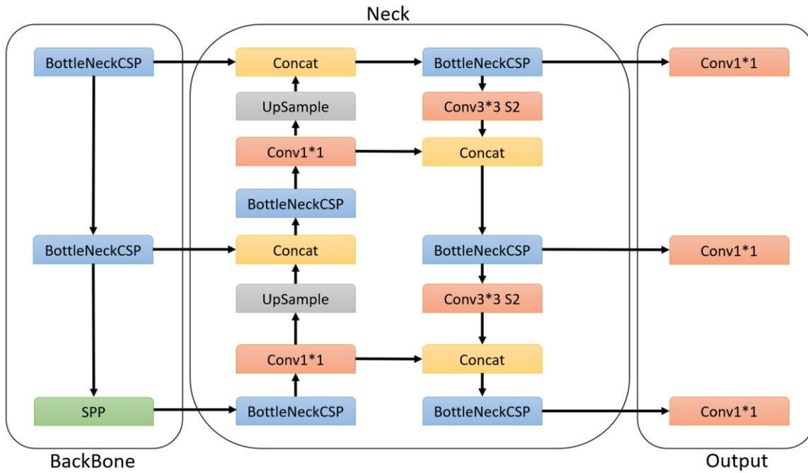
Figure 1. YOLOv5 architecture
