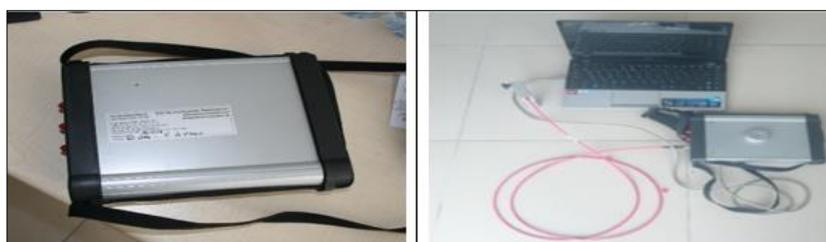
Figure 3. Handheld spectroradiometer used for taking canopy level spectral reflection measurements
