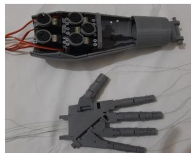
Figure 7. Servo motors located on the robotic
