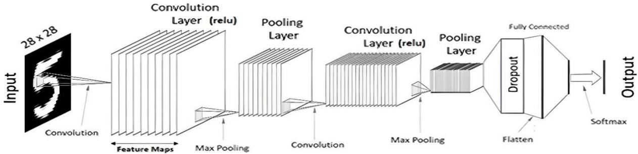
Figure 1. The layer structure of CNN architecture [31]
