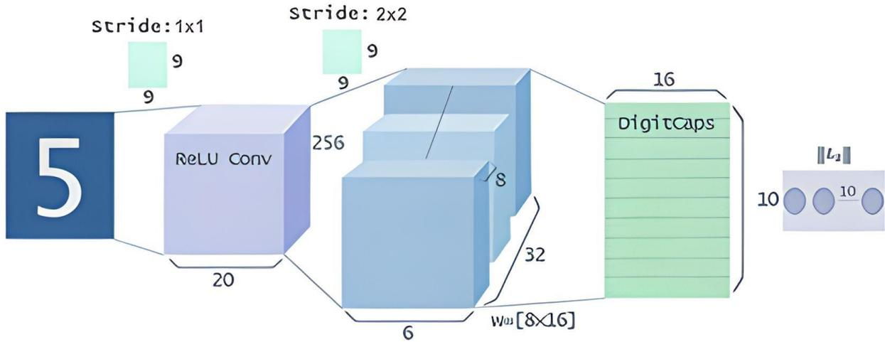
Figure 3. The layer structure of CapsNET architecture [34]
