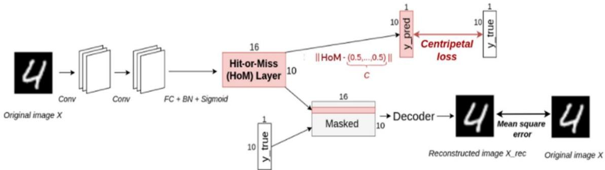
Figure 2. Graphical representation of hitnet architecture [29]
