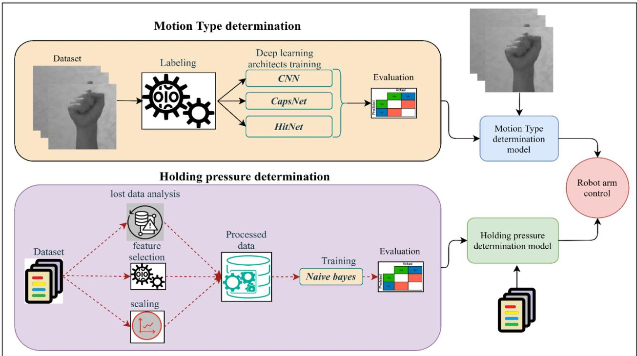
Figure 6. Workflow diagram of hand images and pressure data
