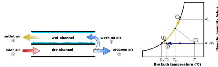
**Figure 3.** M-cycle indirect evaporative cooler [25]
