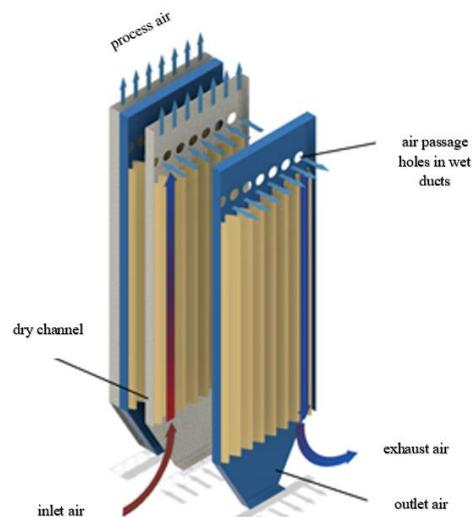
**Figure 5.** Schematic view of the M-cycle heat exchanger
