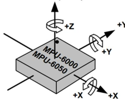
Figure 2. Orientation and polarity of rotation [15]
