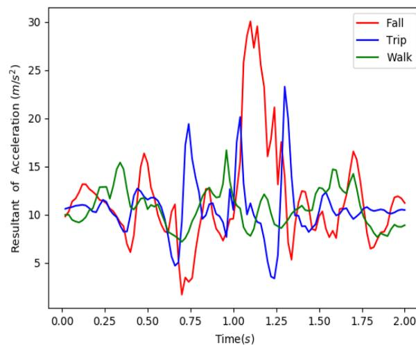
Figure 4. Sample resultant acceleration data
